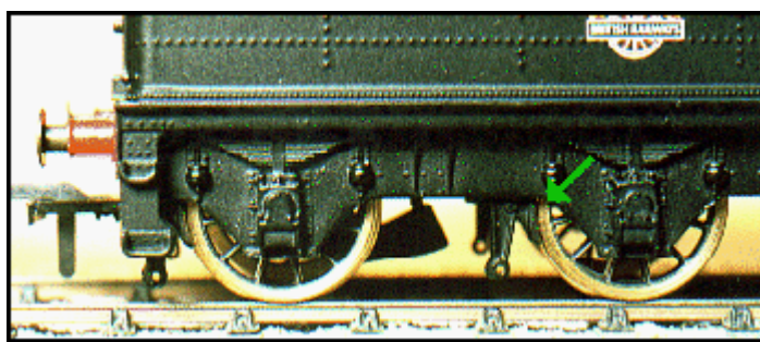
Fig. 6 Ease all brake blocks so they clear wheels.
