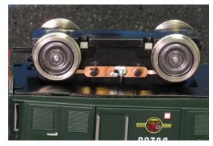
The keeper plate can be replaced, there is an arrow molded on the inner face, make sure that is aligned pointing to the outer end of the locomotive chassis. Make sure two clips on the keeper plate are aligned with the mountings on the bogie chassis, press gently and firmly downwards and the keeper plate will snap into place. Replace the bogie sides and the conversion is complete.
