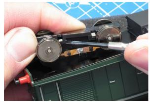
The axles are held in place by a keeper plate on the bottom of the bogie, this can be removed again with a small screwdriver. There are four clips, two per side, which need releasing, and these are on the central section of the keeper plate. Place the blade behind a clip and gently rotate to about 45 degrees or so, and the clip will come free, repeat the process on the same side of the bogie for the next clip. Once one side is undone the clip will lift off allowing access to the gear train.
