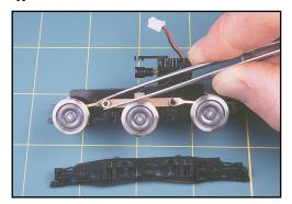
A consequence of the too narrow fitting of the cosmetic bogie sideframes is the lack of room for EM and P4 wheels. Ultrascale supply simple bushes with their wheels to overcome this problem. Slip them over the spiggots before refitting the sideframes.
