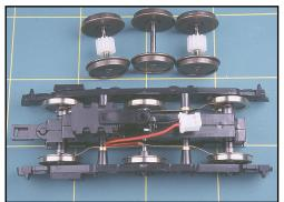
The classic comparison between OO gauge and P4 wheels, the finer appearance of the Ultrascale wheels is apparent. Each Ultrascale wheel set axle is supplied with a metal drive gear compatible with those in each bogie.
