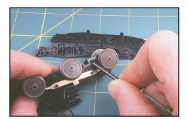
Each bogie is relatively easy to remove from the model without de-soldering leads - the drive shaft just drops out and the lead plug is released carefully from its socket. However it is hard to locate the end of the drive shaft back into the universal joint at the same time as refitting the bogie. A wheel change can be undertaken with the bogies and body left in place. Simply turn the model upside down in a cushioned cradle of some description and pull the bogie sideframes off their spiggots.
