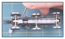
The new wheels simply drop into place. Each is insulated from the axle so it matters not which way they are fitted. Ensure that the phosphor bronze current pick-ups are correctly positioned against the rear rim of the new wheels by teasing the pick up wipers out with a pair of tweezers.
